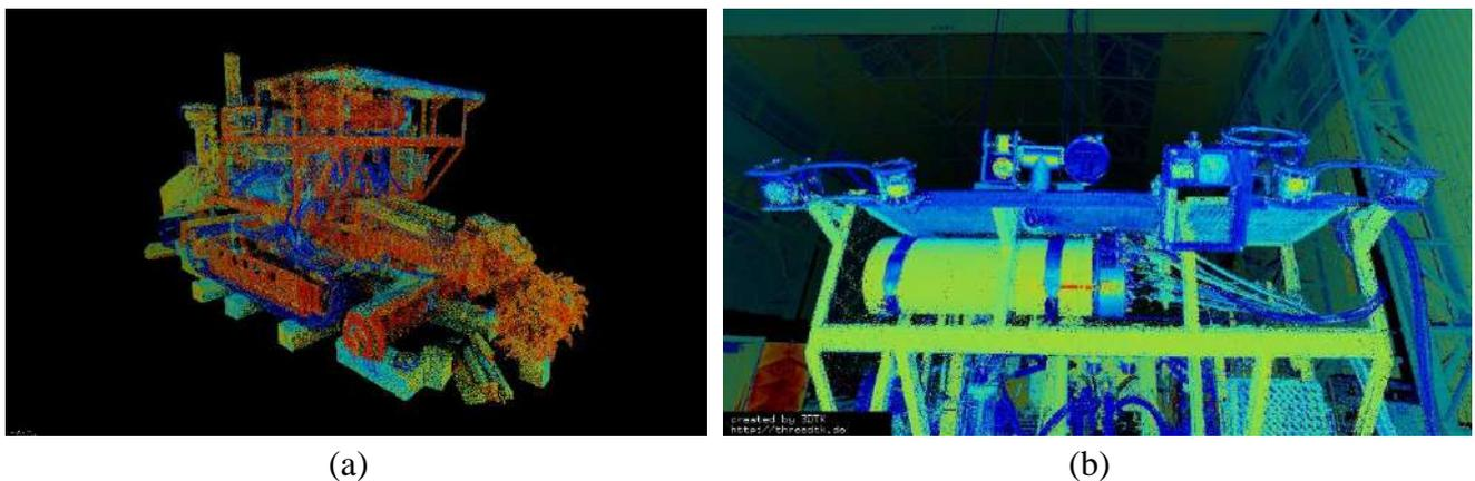
**Figure 2: 3D laser scan of the mining machine (a) and the sensor bar mounted to the vehicle (b). The point clouds are colored by the reflectance values of the laser measurements.**
